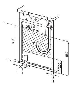
Take into account that it must be possible to pull the appliance forward sufficiently. Ensure the hose does not become trapped when pushing the appliance into position.
